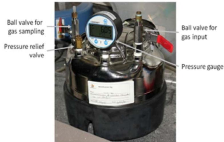
This is a growth chamber. Petri dishes with the bacteria, etc., are placed inside.
