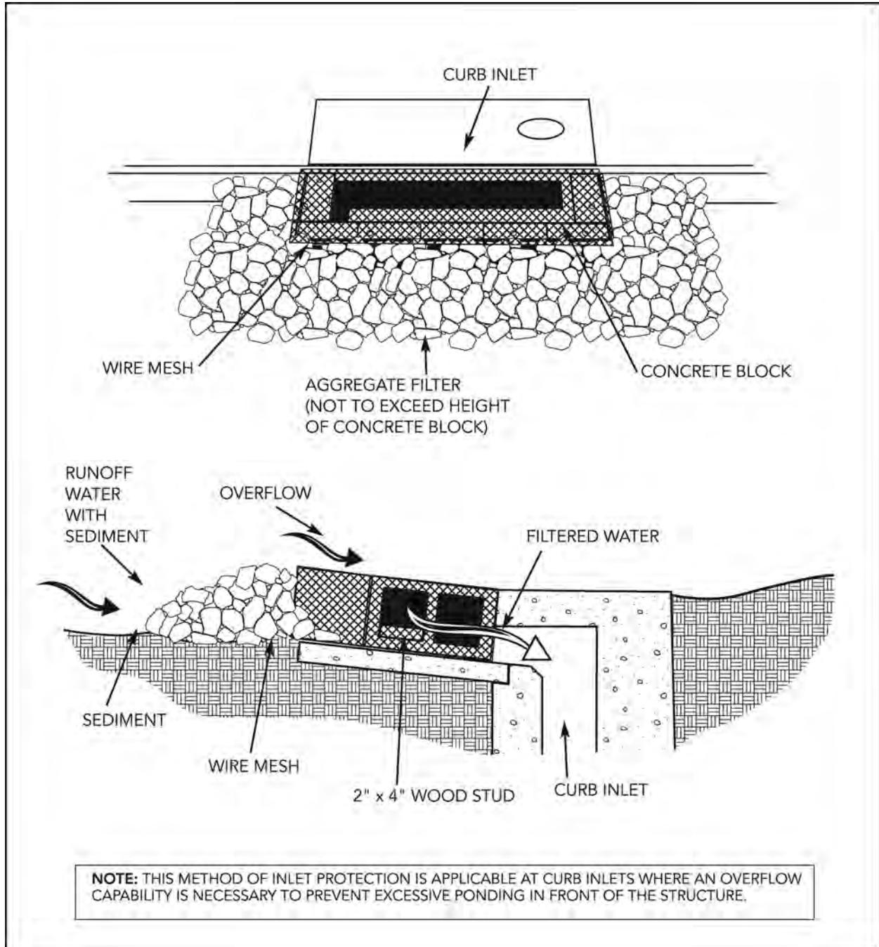
Figure 9-9 Block and Aggregate Curb Inlet Sediment Filter
