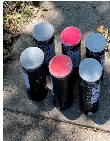
Figure 4: Concrete test cylinders
