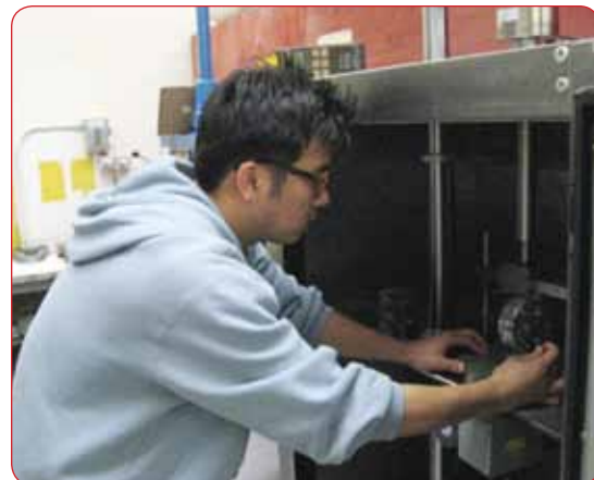
Mr. Soohyok Im, Ph. D student prepares the dynamic modulus test which is one of the most important material properties for the Mechanistic Empirical Pavement Design Guide (MEPDG).
