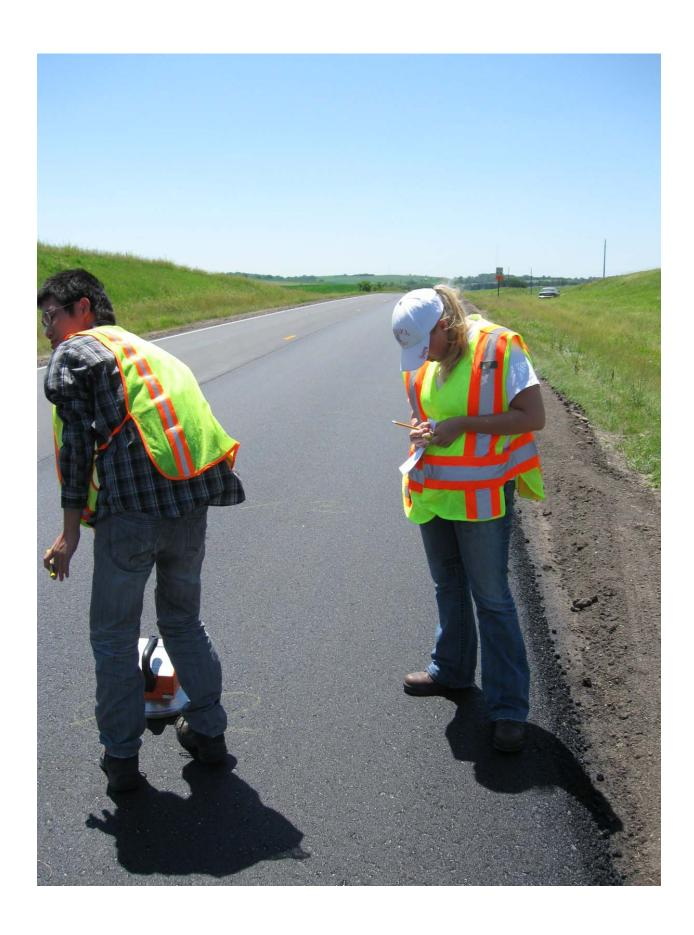
Here I am trying to write down all of the readings Ziquing is taking with the non-nuclear PQI gauge.
