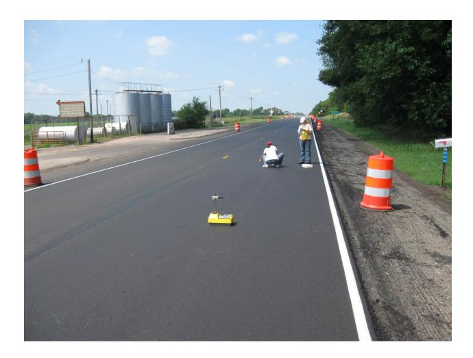
This is a picture of us on a job site in Royal, NE on highway 20. The nuclear gauge is shown in front (the yellow instrument) while Heejung and I take readings with the non-nuclear PQI gauge.
