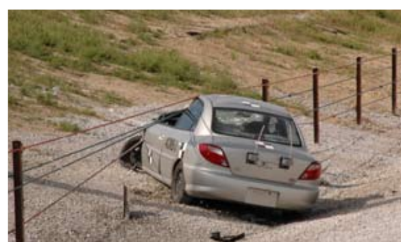
Crash test results on cable guard rail.
