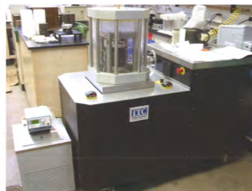
Simple performance testing equipment used to measure the dynamic modulus and flow number of WMA mixtures.
