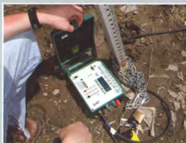
Detail view of a traffic data collection unit.
