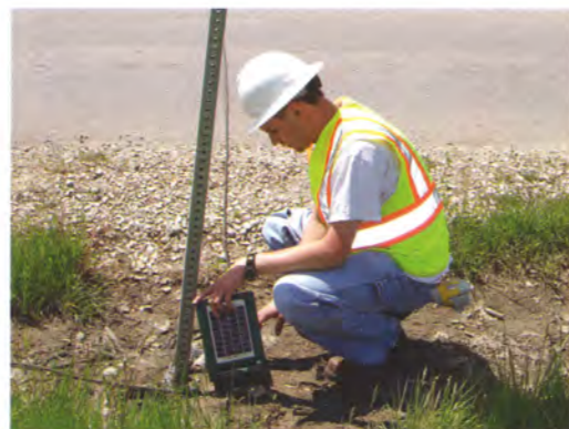
A traffic data collection unit is used to determine the amount of truck traffic passing through Gardner before and after the opening of the intermodal facility.
