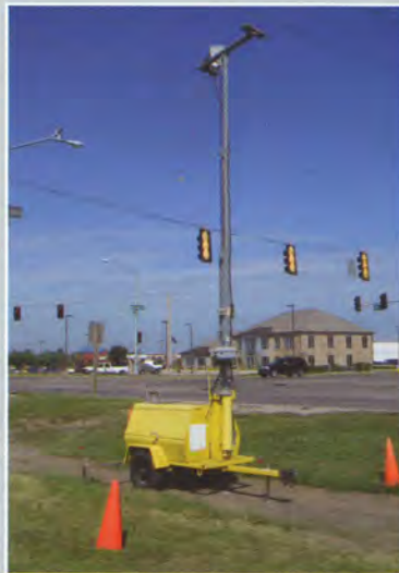
A collection trailer taking video and air quality data in Gardner, KS.
