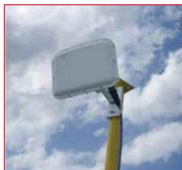
Smart sensor for determining truck speed.
