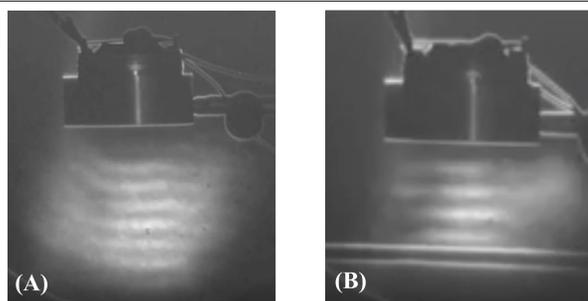
**Figure 2:** Using schlieren imaging we can see sound waves, which are varying pressure waves. This is done by having the flashlight strobe at the same frequency of the sound wave, allowing the camera to always see the same spatial pattern. (A) traveling sound wave; (B) standing sound wave.
