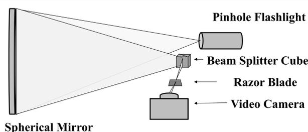
**Figure 1:** Schlieren imaging system setup, which is used to see the varying pressure of air (air flow).
