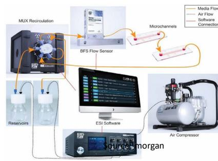
**Fig. 1:** Set-up of the microfluidics system labeled with different components
