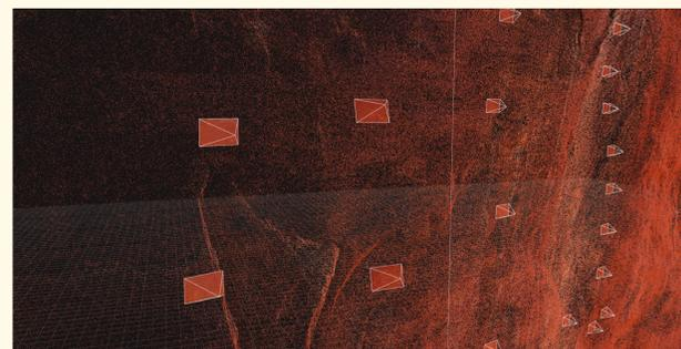
Image 4: Photogrammetry processing steps involving aligning the images and producing the pointcloud
