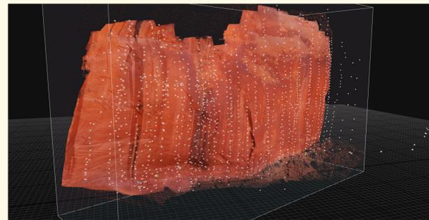
Image 3: Small white shapes show the position and orientation of a photograph captured by the drone
