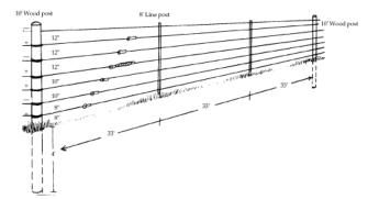
Figure 9. Recommended high-tensile vertical electric fence (Image courtesy of ICWDM).
