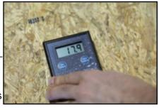
Signal penetration for these types of meters typically ranges up to 1 inch. The meter can be moved across the surface to identify elevated areas of moisture. It is relatively unaffected by temperature and rough surfaces. Measurements can also be taken through coating, varnishes or paints without damage to the surface. Grain orientation does not affect readings.
