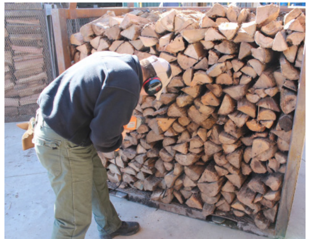
Temperature probe being installed in firewood.
