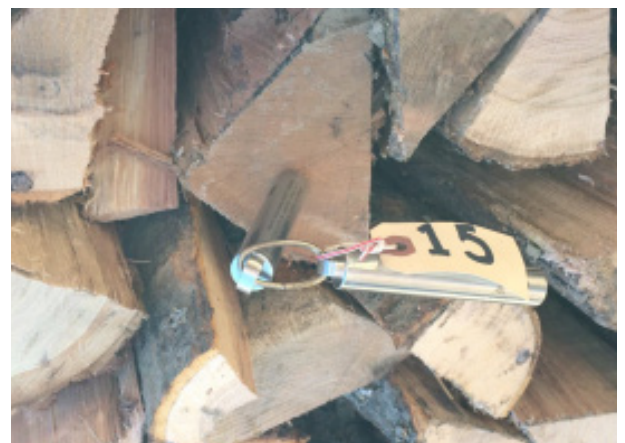
Installed temperature. Several will be installed per kiln load.
