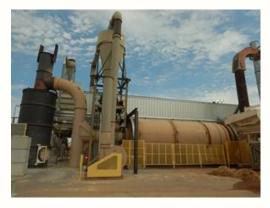
The boiler that heats the dryer runs off sawdust. The triple pass drum dryer weighs 60 tons that has a fan at the end "sucking" material down as it dries.
