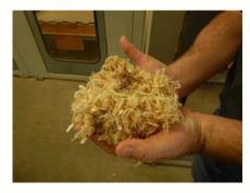
AWF shaves 100 tons of logs per day, each log yields about 50-60% dry fiber after the bark and moisture is removed.
